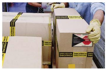
When used in conjunction with companion tools, ShockWatch labels are a deterrent to product mishandling during the transport process as they determine when a sensitive device may have been dropped or bumped within a facility, on a dock or by material handling equipment such as a forklift.
